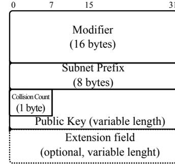
Fig. 1. Format of the *CGA Parameters* data structure
