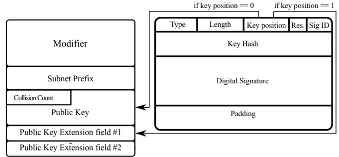
Fig. 4. Public key selection mechanism embedded within the *Universal Signature Option*
